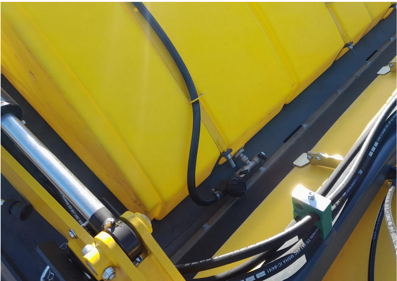
Picture 11. Tank drain valve
