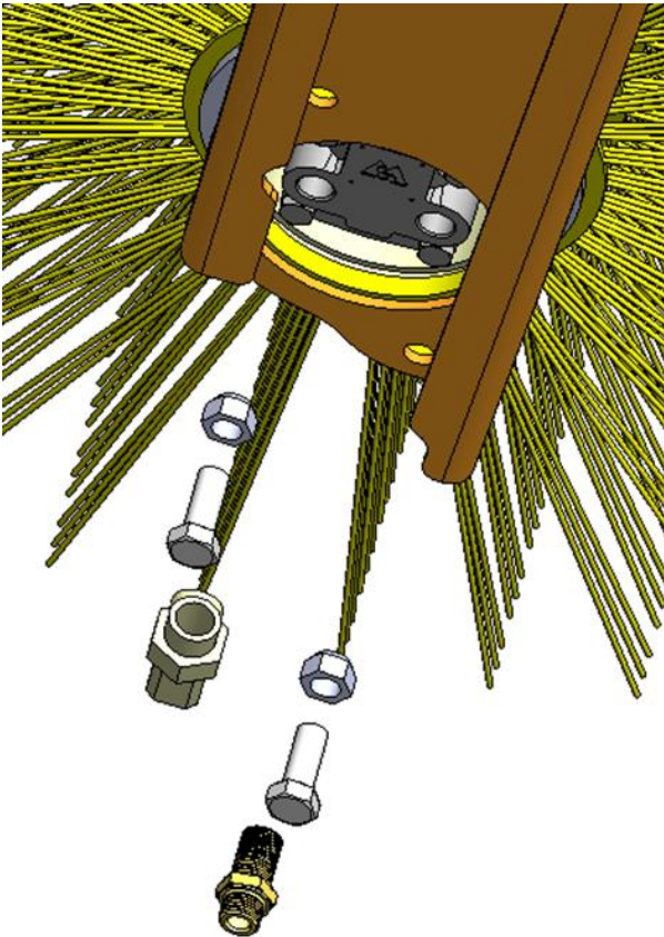
Picture 8. Bolts and connectors on the engine's side
