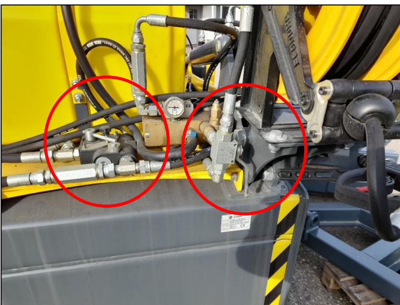
Picture 13. Pump flow control valve and 3-way tap
